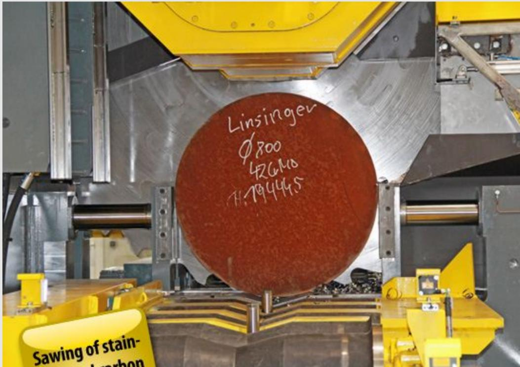
**Sawing of stainless- and carbon steel with only one saw blade**
